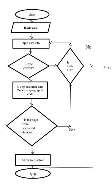
Fig. 1. Flow chart of the proposed 2-factor model using customer registered device
