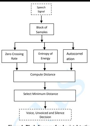
Figure 1: Block diagram of end point detection ([BVN12])
