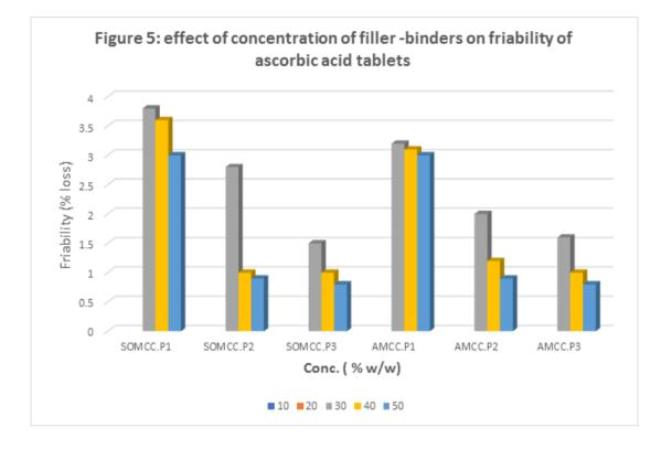
exhibited friability values less than 2%. In these instances, BC's are well over 1000 kgf/m. Interpolation from the graph shows that at 25% w/w of SOMCC or AMCC, BC is more than 900 kgf / m and friability less than 2% for tablet batch made at 93.6MPa. Therefore, a 25-40% w/w composition of these new grades of MCC may be considered optimal for producing acceptable ascorbic acid tablets at compression pressure of between 62.4-93.6 MPa.
