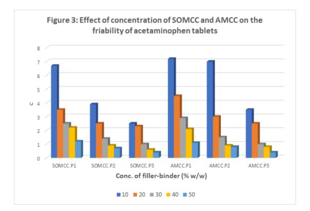
bonding capacity. At polymer concentration of 50% w/w, compact exhibited friability lower than 2% at all compression pressures above 31.2 MPa.
